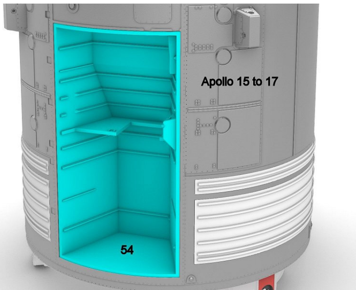
Support structure for the SIM bay
