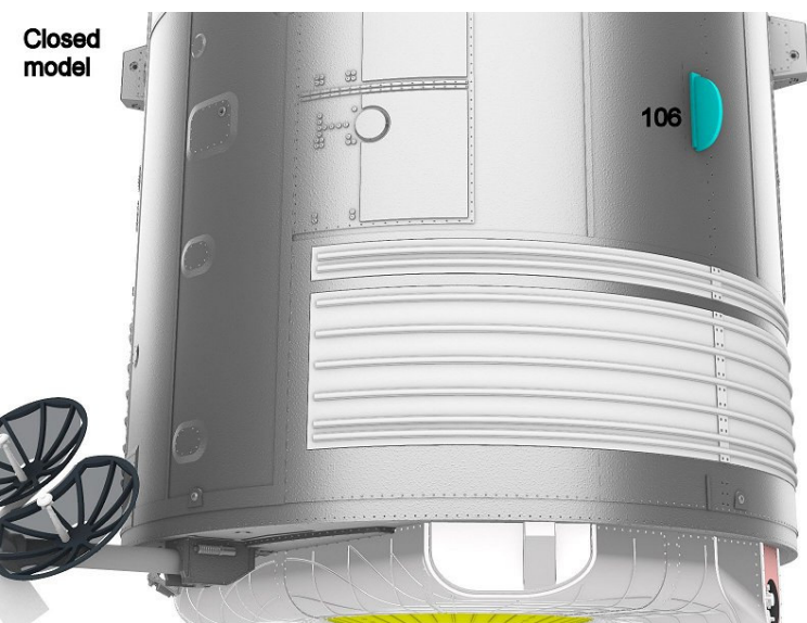
The other scimitar antenna is installed on the other side of the service module.
