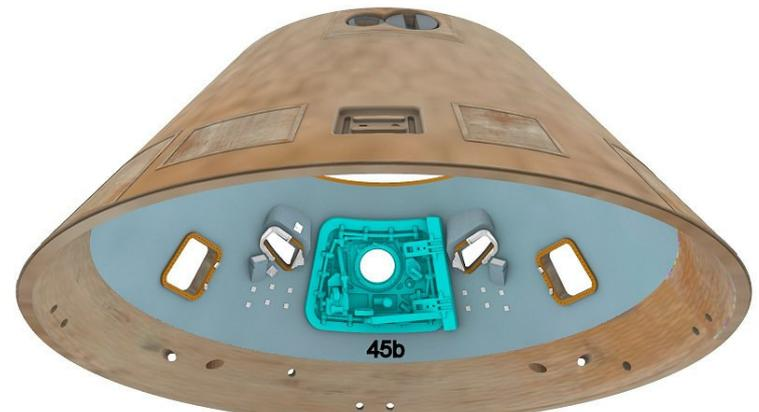
Part 44a1 and subsequent parts 44a2 and 44a3 can be replaced by Part 44a if you have a large printer. If you intend to have a closed hatch, part 45a needs to be replaced by part 45b.
