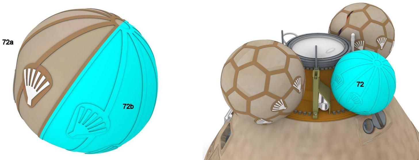
Assembly of the +Z flotation bag.
