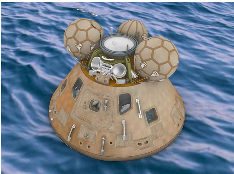
CM just after splashdown, don't forget to add chords between the flotation bags and the parachute section.
