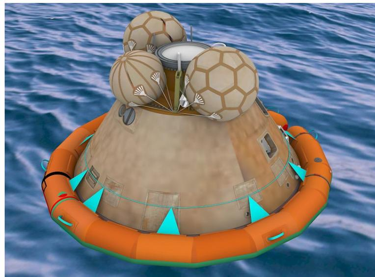
Final assembly of the flotation collar. Isoceles triangles are made out of paper (base 10.5 mm, sides 13,3 mm) as well as handles (width 1 mm).
