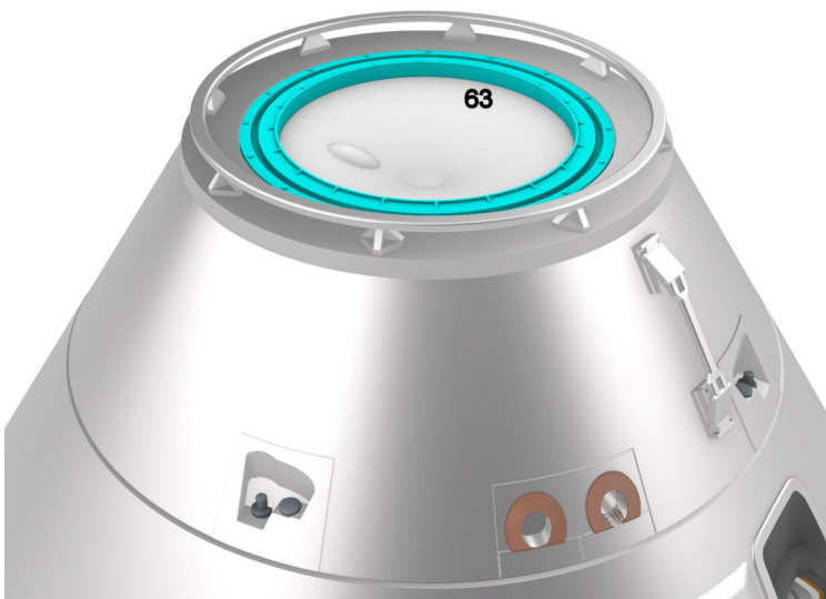
If you intend to represent the CM after the LM was jettisoned or Apollo 7 and Apollo 8 you need part 63 without the docking ring.
