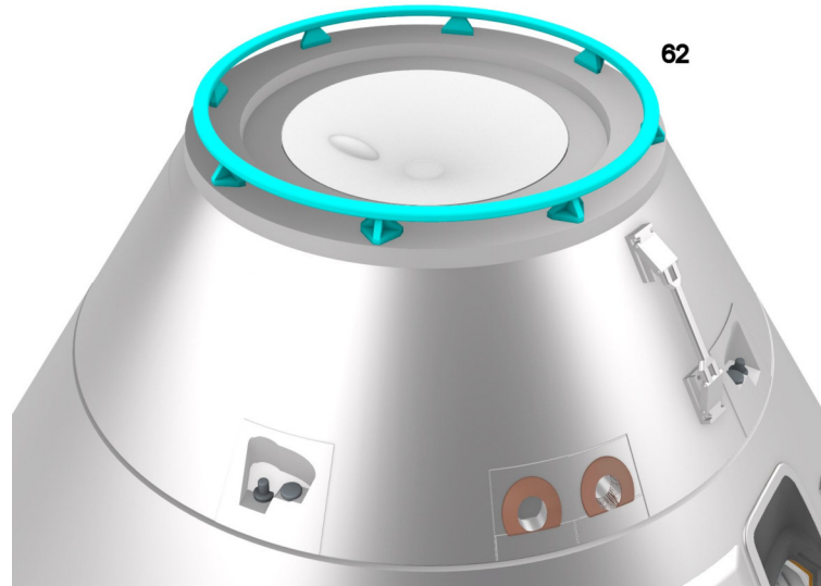
Part 62 is the handle that was meant to be used in case of an EVA transfer between the LM and the CM, it is needed only for Apollo 9 to 17.
